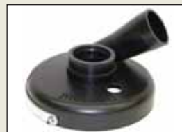
655154000 Dustless 7" Convertable Shroud For concrete surface prep using 7" diamond cup wheels on W24-180, W24-230, W26-230
