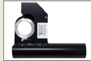
'Dust Director' tuck pointing guard Accepts 4", 4 1/2" 5" and 6" diameter diamond blades. Port is 2". Not for use with Type 1 or Type 27 bonded abrasives. Swivels when approaching an inside corner. (See information under specific model, pages 63-71).
